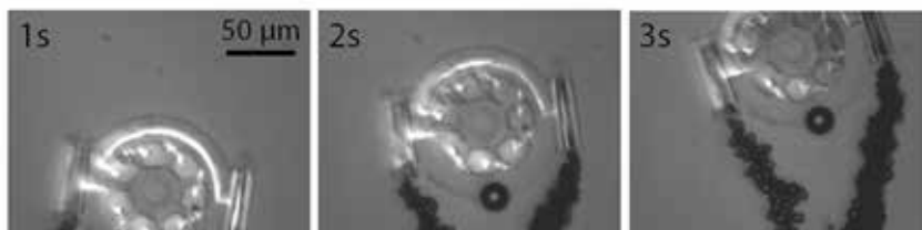
Figure 2: Time lapse of a device swimming under mercury lamp illumination at an air-water interface in 10 mM PBS solution.
