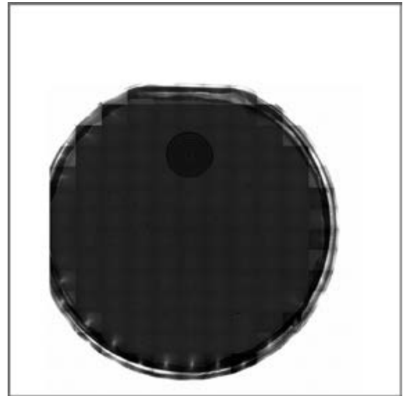
Figure 2: Infra-red transmission image of the two bonded wafers. There is only one bubble of size \sim 4\ \text{cm}^2 . Multiple 1\ \text{cm}^2 samples can be cut from this for further characterization in a Fourier Transform Spectrometer.
