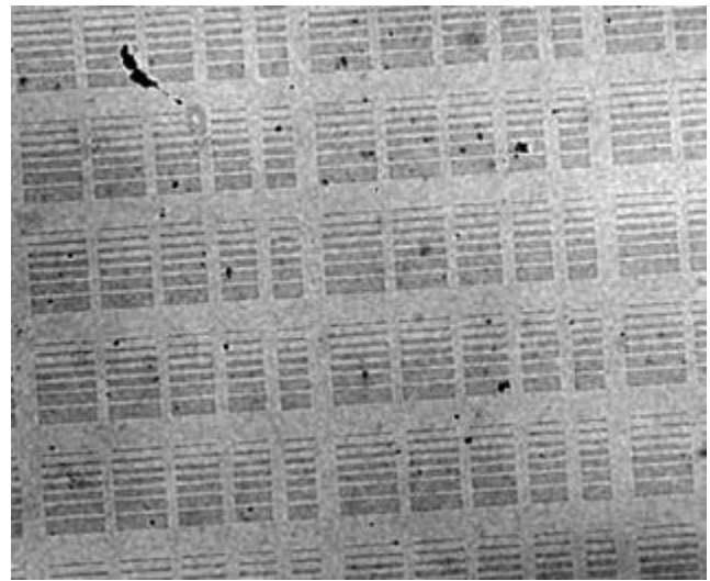
Figure 2: Arrays of graphene bimorph cantilever beams imaged in a transmission optical microscope.
