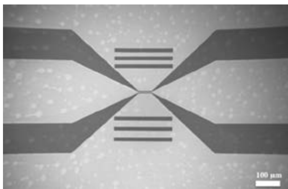
Figure 2: SEM of a fabricated coplanar waveguide. The grid lines above and below the centerline are used to optically locate the center.
