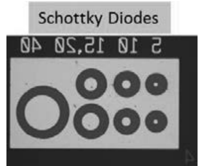
Figure 2: Optical image of circular Au Schottky diodes fabricated on SrTiO 3 /SmTiO 3 /LSAT samples.
