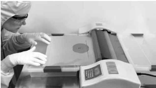
Figure 3: Dry film lamination using an inexpensive office pouch laminator.
