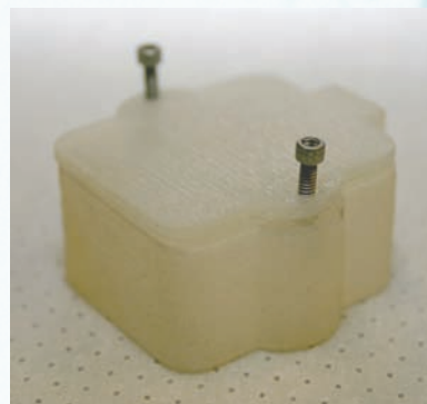
Figure 2: Electrical connection box with threaded screw holes for assembly. Other boxes could be printed in opaque material or painted to restrict the amount of light.
