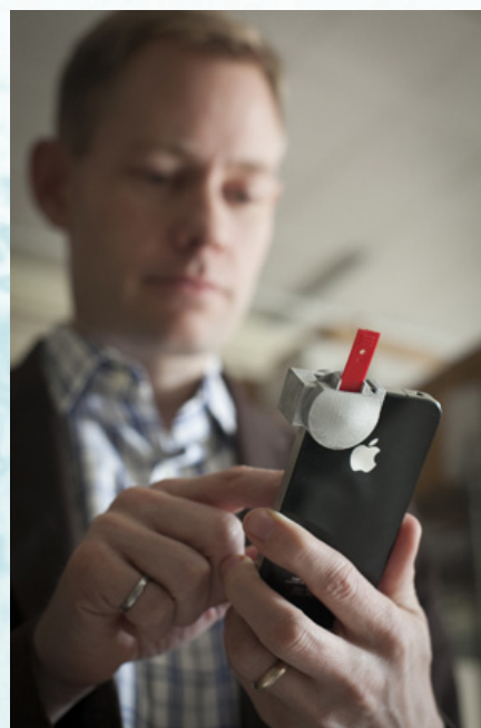
David Erickson, associate professor of mechanical engineering, tests the smartCARD, which uses an application system to read cholesterol levels in about a minute. Jason Koski/UP
