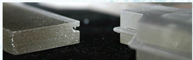
Figure 4: Multi-part device with a tongue-in-groove feature to control the z-axis of the assembled device. These large features and overhangs would require multiple photolithography or machining steps, but they can be printed in a single run on the 3D printer (printed in acrylic-like VeroClear).
