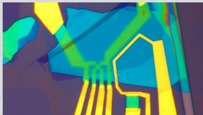
Figure 1: The Nowack Group created this \mu\text{m} -scale Hall-effect sensor by sandwiching graphene between sheets of hexagonal BN, resulting in a device that operates over a greater temperature range than previous Hall sensors. Provided.
