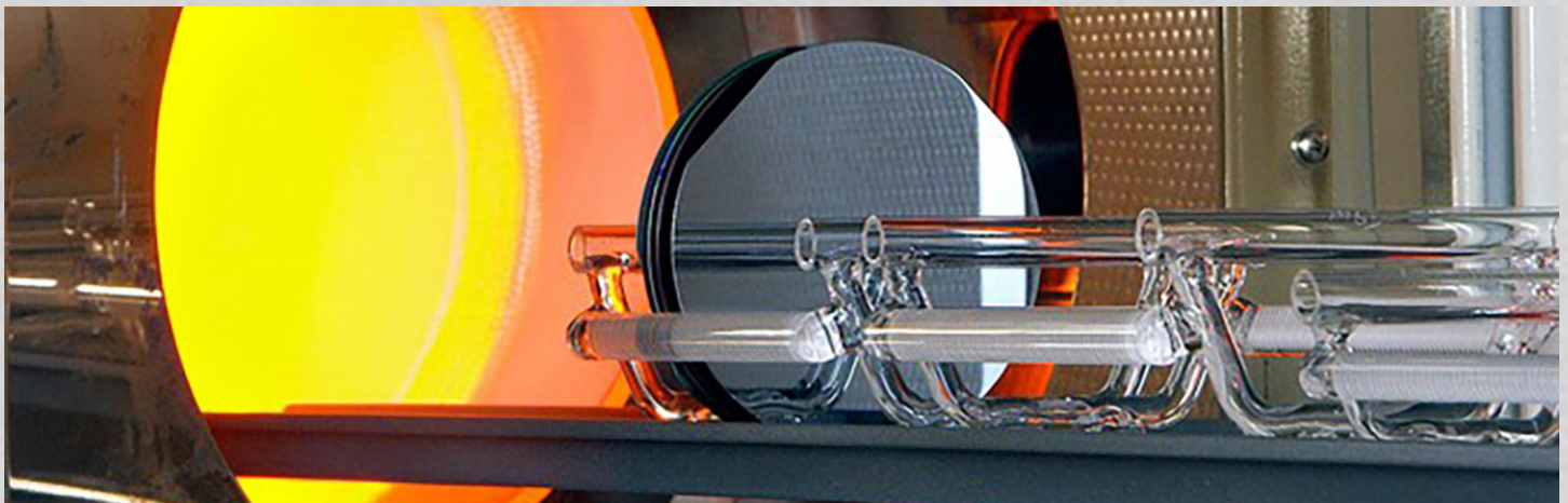
The Cornell NanoScale Science and Technology Facility's Anneal 4 Furnace — an atmospheric furnace with a 40-inch flat zone capable of processing up to 6-inch diameter wafers. Charles Harrington Photography.
