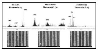
Figure 1: ESI-MS and SEM images after development of different metal oxide photoresists.
