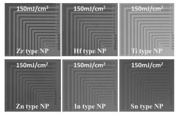
*Figure 3: Optical microscope images of micro-scale patterning using the ABM contact aligner.*
