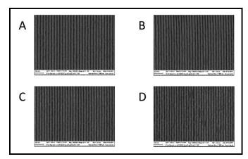
*Figure 4: SEM of EUV exposure results with zinc nano-cluster resist. (A) 16 nmLS with 45 mJ/cm*<sup>2</sup>. (B) *15 nmLS with 47 mJ/cm*<sup>2</sup>. (C) *14 nmLS with 36 mJ/cm*<sup>2</sup>. (D) *13 nmLS with 35 mJ/cm*<sup>2</sup>.
