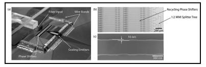
*Figure 1: (a) 512-element silicon photonic array chip wire-bonded to interposer. (b) Microscope image of a section of the array of recycling phase shifters and tree of 1:2 MMI splitters (light flows right to left). (c) Scanning electron micrograph of sidewall grating on 450 nm wide emitter waveguide.*
