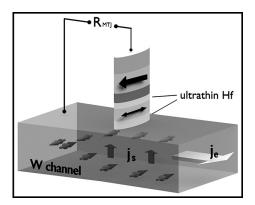
*Figure 1: Schematic picture of the three terminal MTJ and measurement technique.*
