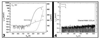
*Figure 3, left:* Representative  $I_d/I_g-V_{gs}$  transfer characteristics in the semi-log and linear scale, along with the extracted subthreshold slope. *Figure 4, right:* Representative three-terminal off-state (at  $V_{gs} = 0 V) I_d/I_g-V_{ds}$  characteristics and breakdown voltage of  $Ga_2O_3$  vertical power MISFETS.
