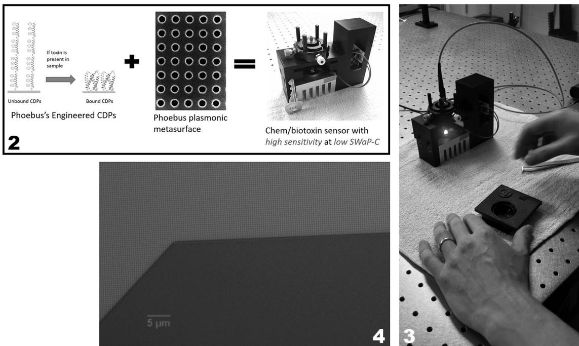
**Figure 2, top left:** Phoebus-engineered sensor system combines; (a) Designed CDPs which undergo extreme conformational changes upon binding target (b) Gold metasurface, patterned to maximize transmission at SPR resonant wavelength into (c) a high sensitivity, low SWaP-C chem/biotoxin sensor system. **Figure 3, top right:** Complete Phoebus handheld biosensor system. **Figure 4, above:** Optical microscope image of a metasurface used in disposable biosensor chip.
