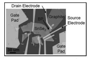
*Figure 1: Optical image of the representative BP/SnSe*<sub>2</sub> *TFET.*
