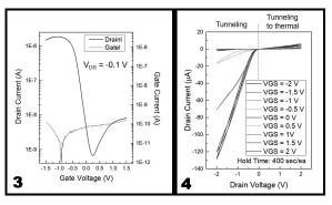
Figure 3, left: Current as a function of gate voltage at VDS = -0.1 V at room temperature in N<sub>2</sub>. The black line indicates drain current and the red line indicates gate leakage current. Figure 4, right: Drain current as a function of drain voltage with different gate voltages.
