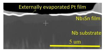
Figure 1: Cross-sectional image of STEM specimens that yield highresolution atomic imaging.
