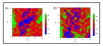
Figure 3: Atomic force microscopy images of  $Nb_3Sn(a)$  before and (b) after laser annealing [8].
