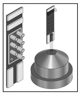
Figure 1: Images of CryoSAXS sample devices. The sample is held in place between two silicon nitride X-ray windows by Kapton<sup>®</sup> tube. The X-ray passes axially through the tubing. Multiple sample cells are present in a single device in two rows. One row contains solutions with a macromolecule and the other is analogous solutions without the macromolecule to be used for background subtraction.
