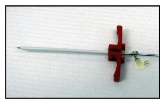
Figure 1: A prototype deep brain insertion sub-assembly is shown which includes a protective split-sheath inserter, the actual electrode array/signal cable and the tungsten insertion rod.
