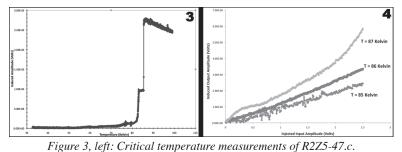
Figure 4, right: Critical voltage measurements of R2Z5-47.c.
