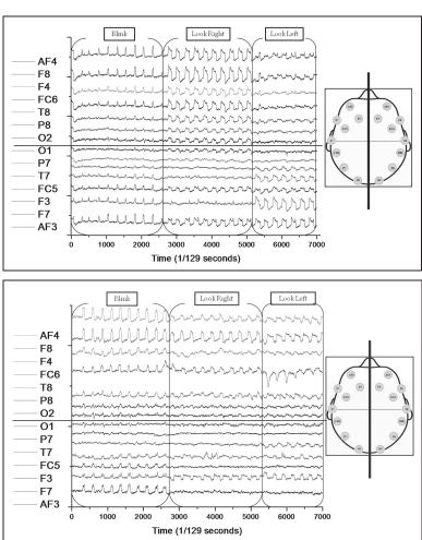
Figure 3, top: Wet electrode EEG results with headset map. Figure 4, bottom: Dry electrode EEG results.
