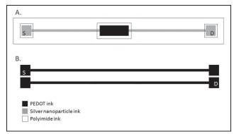
Figure 1: A. Pattern for multilayered OECTs using source (S) and drain (D) silver nanoparticle electrodes, polyimide passive layer, and a PEDOT active site. B. Pattern for all-PEDOT OECT.
