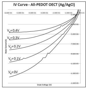
Figure 3: Current vs. voltage graph for all-PEDOT OECT using an Ag-AgCl gate electrode. The gate voltage  $(V_g)$  is applied between 0.0V and 0.4 V at 0.1V intervals.
