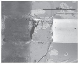
Figure 2: The silver nanoparticle electrode on the multilayered OECT after exposure to electrolyte and degrading. The silver nanoparticle ink has been removed between the PEDOT:PSS layer (left) and the polyimide layer (right).
