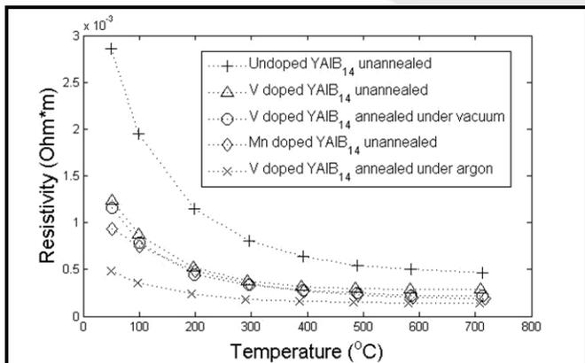
Figure 1: Resistivity of vanadium and manganese doped samples. Most samples had similar resistivities. Undoped YAIB<sub>14</sub> had high resistivity, and vanadium doped YAIB<sub>14</sub> annealed under argon had low resistivity.
