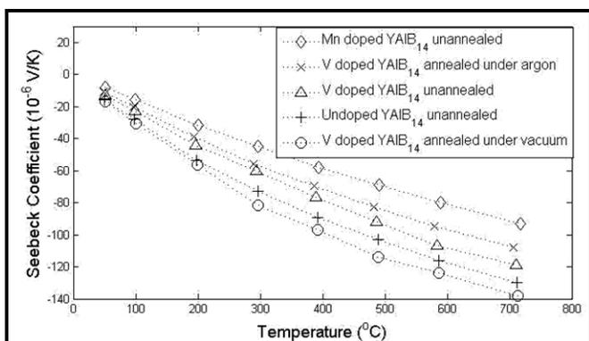
Figure 2: The Seebeck coefficient of vanadium and manganese doped samples. The lowest Seebeck coefficient belongs to manganese doped YAIB<sub>14</sub>, and the highest is vanadium doped YAIB<sub>14</sub> annealed under vacuum.
