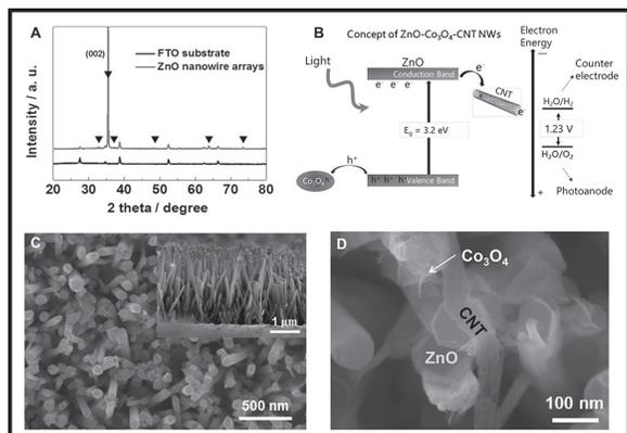
Figure 2: (A) XRD pattern. (B) Bandgap concepts. (C) ZnO NWs. (D) ZnO-Co<sub>3</sub>O<sub>4</sub>-CNT NWs.
