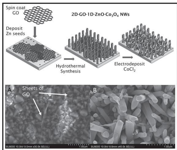
Figure 4: GO-ZnO-Co<sub>3</sub>O<sub>4</sub> NW synthesis. (A) GO on FTO. (B) ZnO on GO-FTO.
